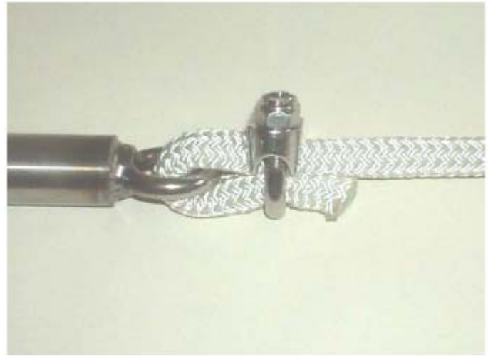
6. Attaching the tow rope to the turbine
