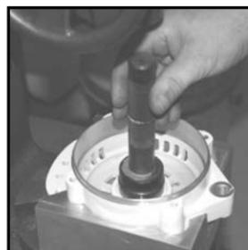
**14. Installing Rear Bearing**
