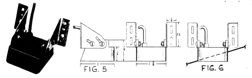
Holding the transducer and bracket in the position required, mark its location. Mark and drill four mounting holes. Use four stainless steel screws or bolts to mount the bracket. Install the transducer. Drill a 7/16" hole well above the water line to route the transducer cable into the boat.
