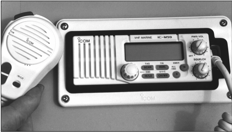
ICOM's IC-M59 VHF set is shown with optional flush mount kit.
