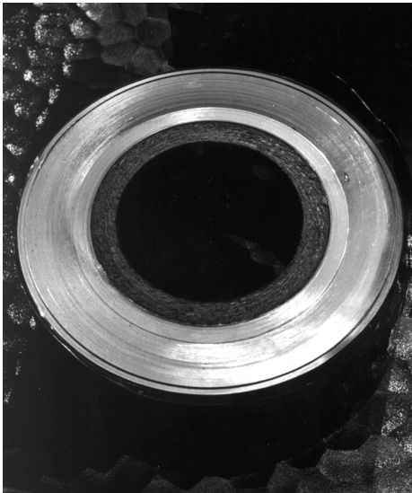
Use 3-inch wide, 3-mil copper foil to ensure a good sea water ground.
