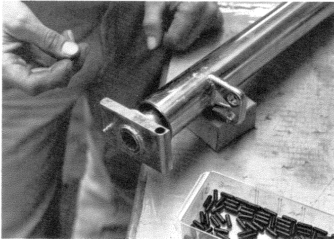
Loading rollers into lower strut bearing.
