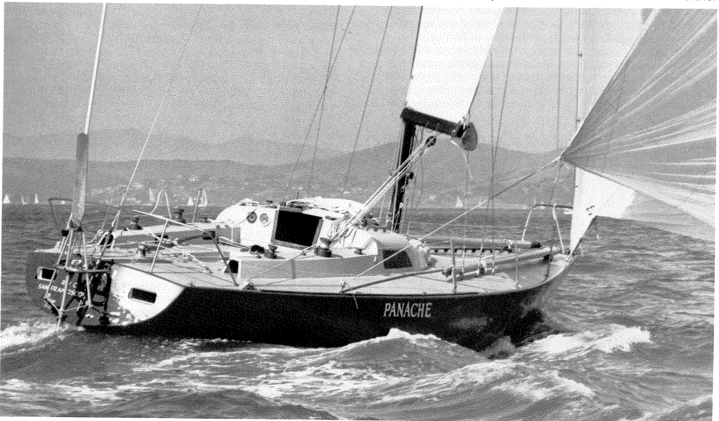
PANACHE, a 40' ultralight displacement racer, was the fastest monohull in the 1980 single-handed Trans Pacific Race. Using elastic cord limiters as discussed in 4.5.3 the MONITOR was made to steer under spinnaker for hours on end, even with the boat surfing.
