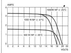
The IV curve (current vs. voltage) above demonstrates typical power response to various light levels at 25°C and a 47°C cell temperature.
