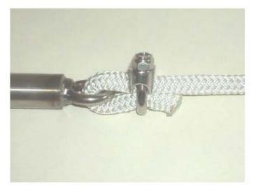
5. Attaching the tow rope to the drive coupling
