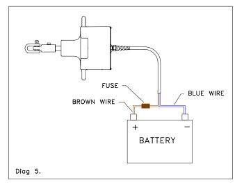
The BROWN WIRE is connected to the POSITIVE + terminal and the BLUE WIRE to the NEGATIVE - terminal. **VERY IMPORTANT**. BE CAREFUL, AS INCORRECT CONNECTION WILL DAMAGE THE RECTIFIER. WARRANTY WILL BE DISCLAIMED.
