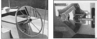
These photos show the simplicity and utility of a Rack and Pinion Installation. Cover box makes an excellent helmsman seat with a hinged top for quick maintenance and inspection.
