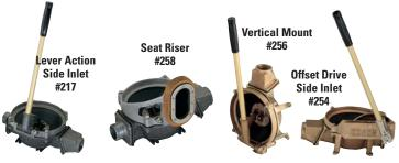
**18GPM Manual Diaphragm Pumps** are offered in varying configurations to facilitate installation based on where you want to locate the pump on the boat. The #254 Offset Pump facilitates mounting the pump behind a bulkhead, the #256 Vertical Mount Pump allows mounting the pump on a wall and the #258AL is ideal for mounting behind a set riser in the cockpit. An 18" aluminum handle comes with every pump. A 32"/81cm handle, available in plated or stainless steel is optional.
